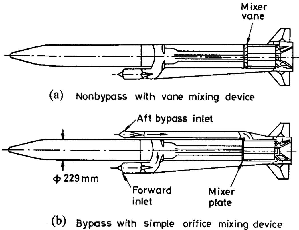
Fig. 3 Solid fuel ramjet powered missiles.<sup>20</sup>
