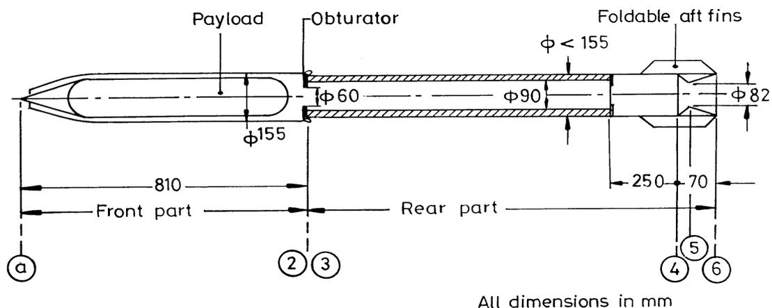
**Fig. 1 Gun launched SFRJ-powered projectile.**
