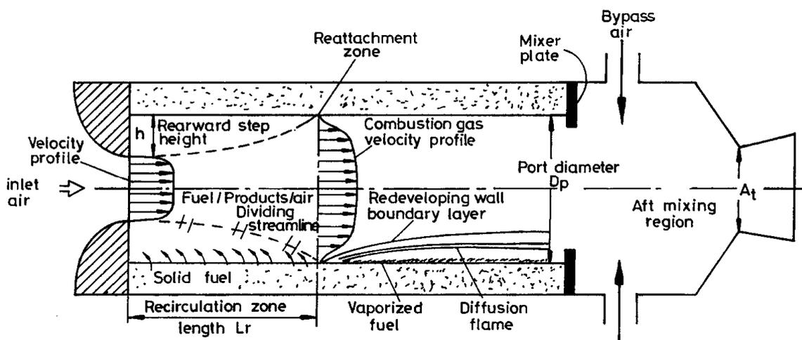
Fig. 2 Combustion chamber flow field in a solid fuel ramjet.<sup>10,11</sup>
