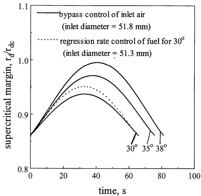
**Fig. 11** Inlet operation under bypass control of inlet air. The fuel grain length is 1070 mm, the nose ogival slenderness ratio is 2.5, the annular gap is 6.5 mm, the constant A in the regression rate equation is  $8.5 \times 10^{-3}$ , and the throat diameter is 82 mm.
