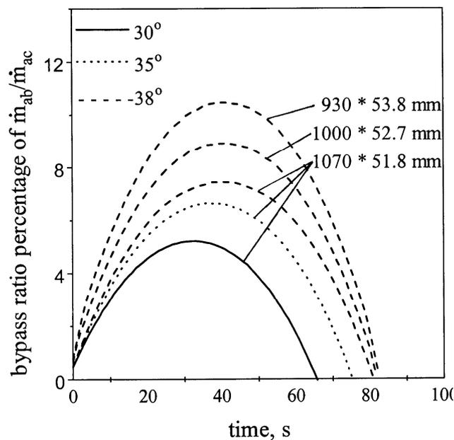
**Fig. 9 Percentage variation of bypass ratio of inlet air. The nose ogival slenderness ratio is 2.5, the annular gap is 6.5 mm, the constant A in the regression rate equation is  $8.5 \times 10^{-3}$ , and the throat diameter is 82 mm**
