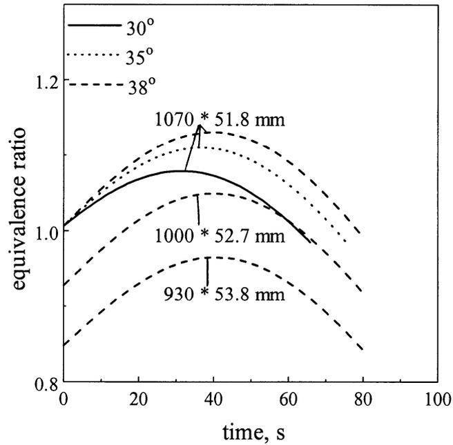
**Fig. 10** Equivalence-ratio variations under bypass control of inlet air. The nose ogival ratio is 2.5, the annular gap is 6.5 mm, constant A in the regression rate equation is  $8.5 \times 10^{-3}$ , and the throat diameter is 82 mm.
