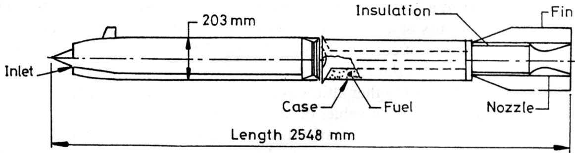
**Fig. 5 SFRJ assisted 203-mm M110A-2 cannon launched projectile.<sup>16</sup>**
