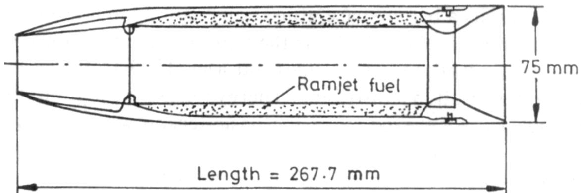
Fig. 4 SFRJ-assisted 75-mm gun launched projectile.<sup>16</sup>
