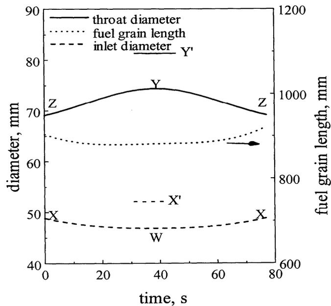
**Fig. 8** Variation of fuel grain length, throat diameter, and inlet diameter. The launch angle is 35 deg, the nose ogival slenderness ratio is 2.5, the annular gap is 6.5 mm, and the constant A in the regression rate equation is  $8.5 \times 10^{-3}$ .
