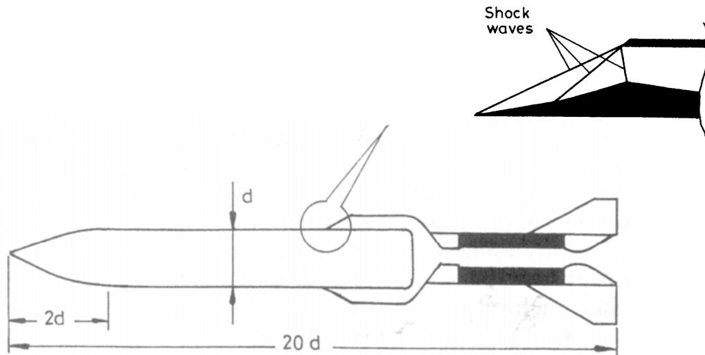
**Fig. 7 Geometry of the high speed air-to-air missile.<sup>7</sup>**
